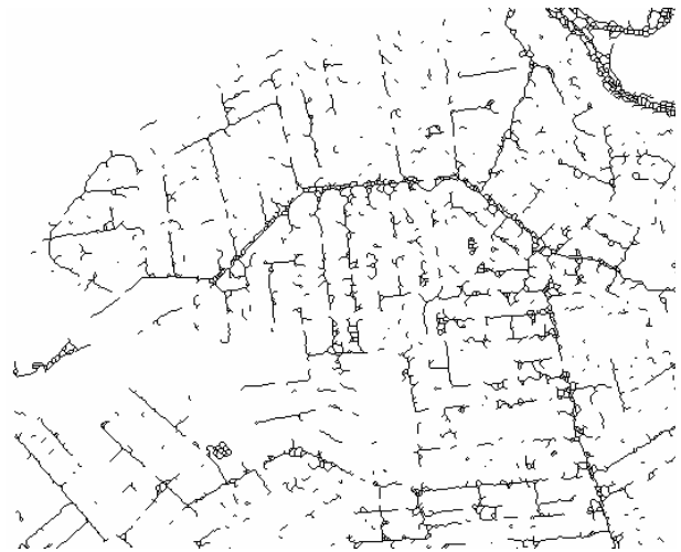
Figure 5. Results of detected roads. This output result has been thinned with a threshold of 5 pixels in noise removal and a threshold of 4 pixels in road segment joining.
