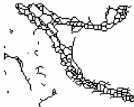
Figure 6. An enlarged portion of the extracted road network. Road segments shorter than the removal threshold after thinning have not been removed. Roads wider than one pixel in the input image have some branches on the edge and appear as a web inside.
