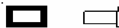
Figure 7. A rectangular road block and its thinned output. The output contains two tiny branches because of the sequence of iteration. They will shift to the left if the order of iteration is reversed.
