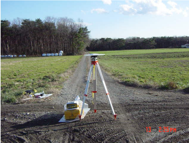
Photo 1. Example of static GPS measurement in Tochigi area
